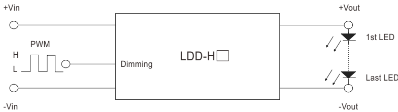
Fig-1 12VDC input, 1~3 LEDs(Vf=3V)
