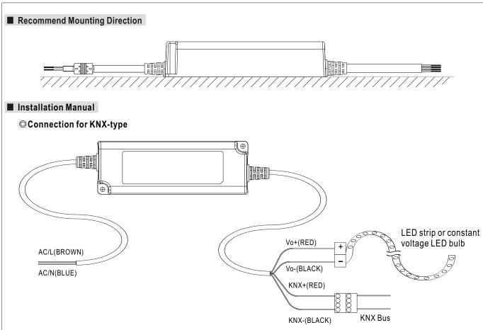
PWM KN series can be ETS adressing/programming WITHOUT connecting to AC mains
