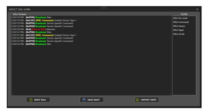
Once connected, use the ADDICT Sniffing Menu to open the dialog shown above. The information can be saved to file, and also filtered for specific actions.
